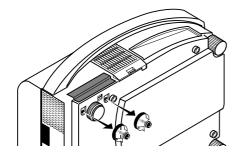
3. Remove the slot cover by pushing up on the catch of the cover with a flat-head screwdriver until you feel it detach.
